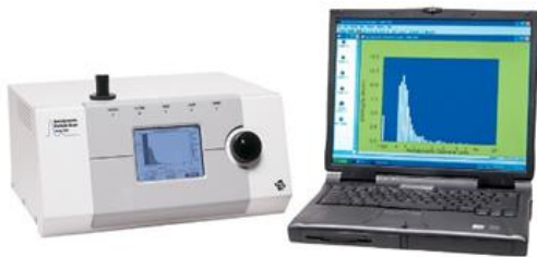
Figure 5. TSI Aerodynamic Particle Sizer (APS) model 3321 used to measure total particle concentration and particle size distribution of the challenge bioaerosol. Range 0.54-20.0 \mu\text{m} aerodynamic diameter, with 1 particle/L detection limits.
