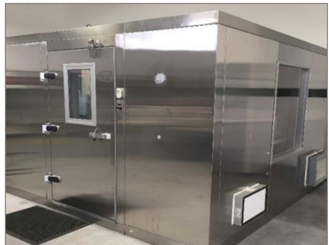
Figure 2: Stainless Steel Bioaerosol Test Chamber used for all Violet M Testing. The chamber is equipped with HEPA filtered air (in/out), multiple bio aerosol sampling ports, decontamination, and pressure balance. Exterior picture.
